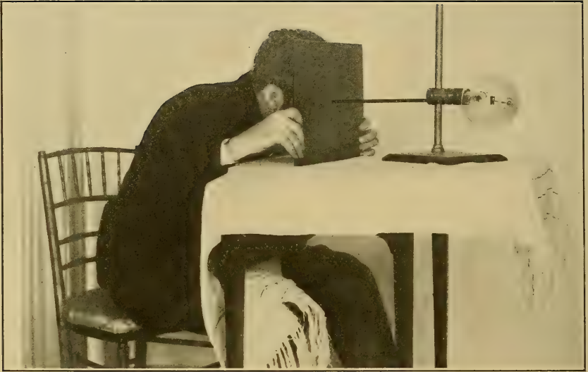
PLATE 54.—Author's Position Finder. Sighting through channel of rod to find axis of rays from the tube-focus. See text for full description of method.
